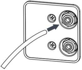
**Connect** water line to water inlet connector at back of unit. (See manual if installing filters)
