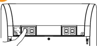
**Switch** water source switch on left side from "Bottle" to "POU".
