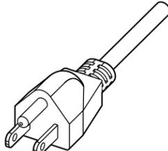
**Plug** cord into a grounded GFCI outlet.
