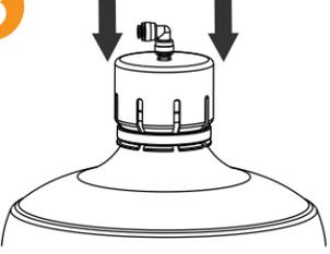
**Insert** Cap with siphon tube into the water bottle.
