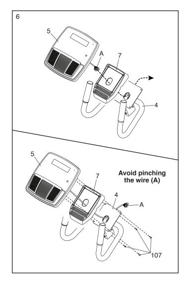
7. While a second person holds the Console Bracket (4) near the Frame (1), connect the wire (A) on the Console (5) to the Main Wire (115).
