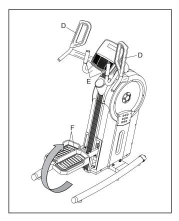
To dismount the trainer, wait until the pedals (F) come to a complete stop. Note: The trainer does not have a free wheel; the pedals will continue to move until the flywheel stops. When the pedals are stationary, step off the higher pedal first. Then, step off the lower pedal.
