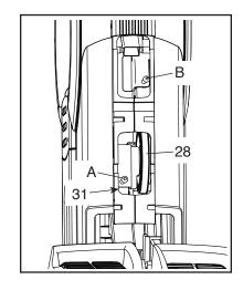
Stand on the trainer and pedal for a few moments. If the pedals still slip, step off the trainer and locate the upper Adjustment Screw (B). Tighten the upper Adjustment Screw two turns; this will tighten the Small Drive Belt (28).
